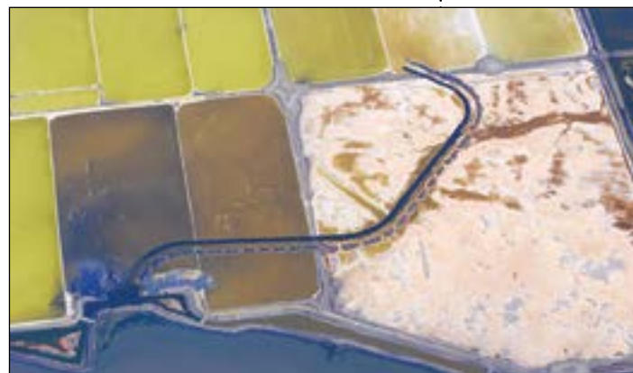
Recycled water isn’t just for irrigation. When this former Cargill Salt property in the North Bay was restored, beginning with excavation of the historic slough as shown above, a new pipeline brought recycled water in to dilute the toxic residue left behind by salt processing. The pipeline will continue to provide 1,700 acre-feet of recycled water per year to the former bittern ponds (potable water would have been prohibitively expensive). In the East Bay, Hayward’s Ora Loma Sanitary District has offered recycled water to help restoration engineers recreate the natural freshwater seeps that once bordered marsh systems. Photo courtesy Russell Lowgren.
