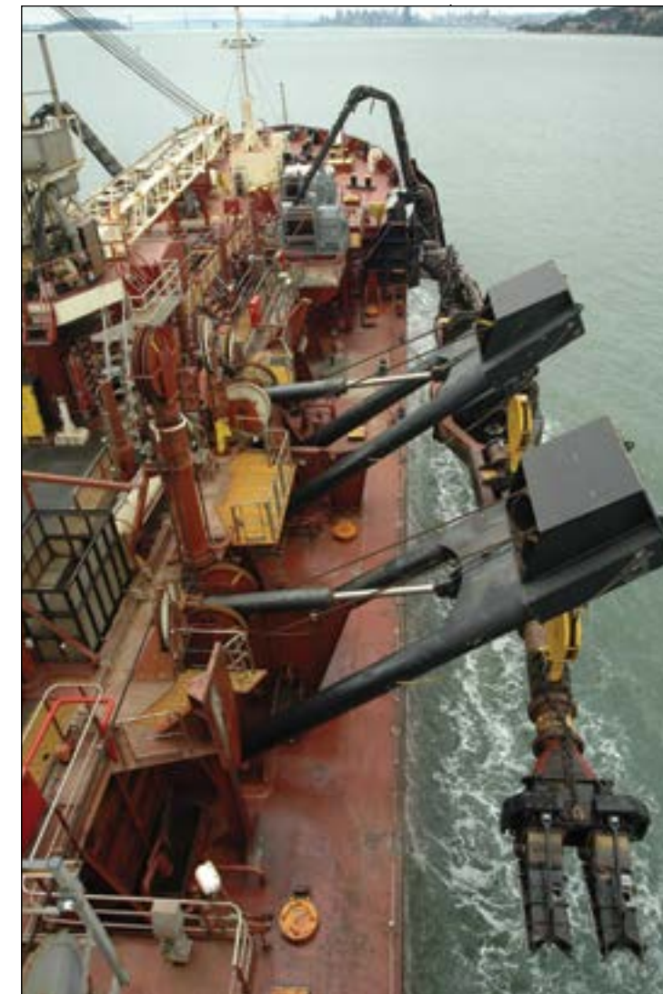
Referred to as a suction hopper dredger, Essayons is able to vacuum up nearly 6,000 cubic yards of ocean sand in one hour using its two drag arms. Photo courtesy USACE.
