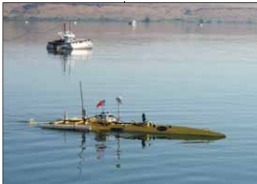
USGS also uses robot boats to monitor flows. The ten-foot-long-length of these boats, which are equipped with acoustic Doppler current profilers, enables them to span the 4-5 foot wave lengths common in wide delta channels without bobbing. The robot boats also maintain a much steadier course than any heavier, human-controlled vessel.
