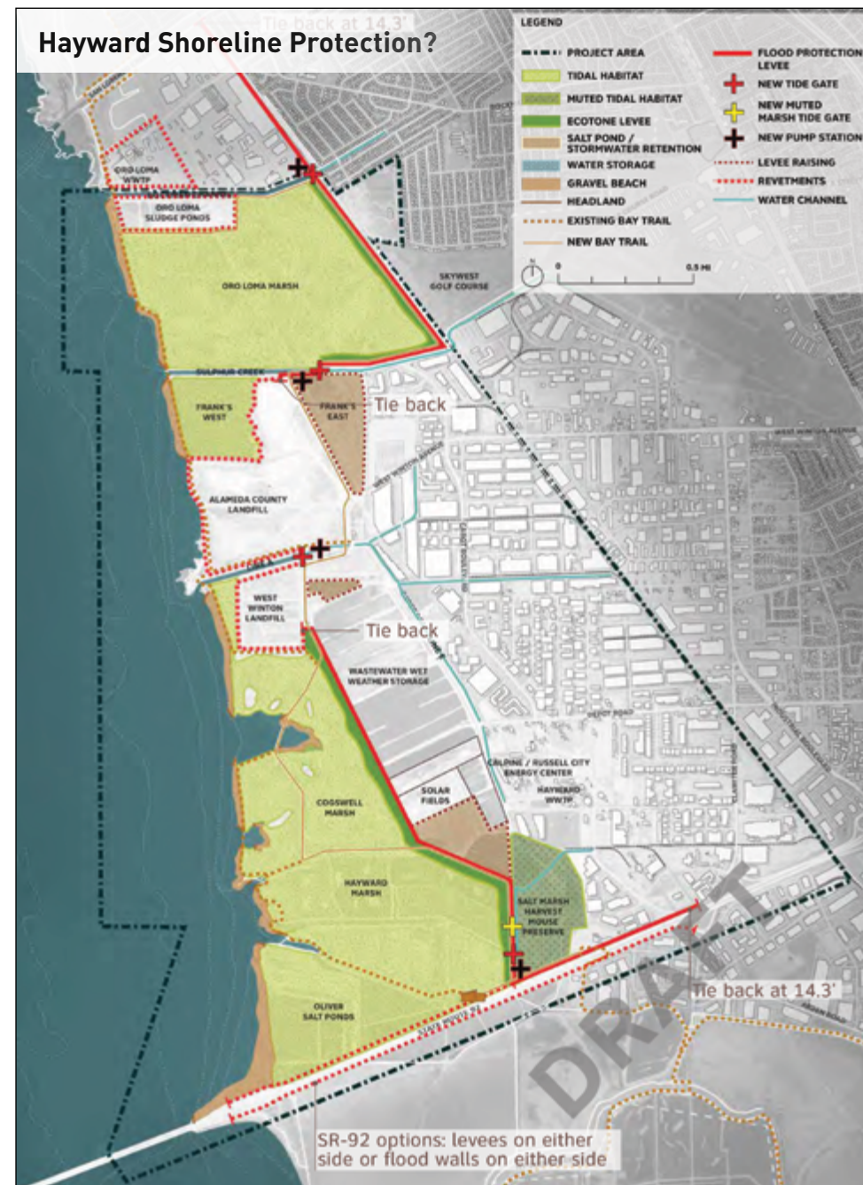
"Down the Middle" line of flood protection. One of three options in the Hayward shoreline adaptation plan. Map: SCAPE
