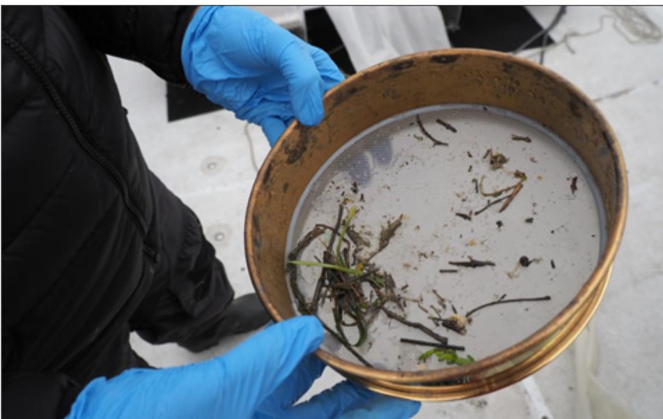
Sieve used to find microplastics in runoff. Photo: SFEI
